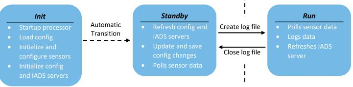
Upon receiving power, the PDAS automatically transitions through the initialization state and enters the standby state. In the standby state, all of the software modules are active except for datalog. In this state, you can view PDAS data via the web server or IADS server, modify the PDAS configuration, and download or delete data log files from the PDAS storage.
