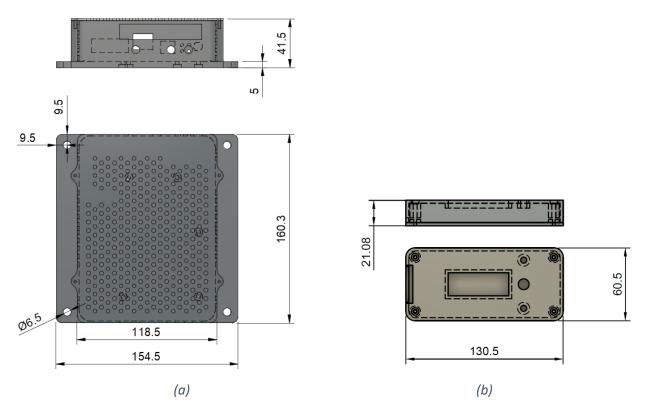
Figure 3: PDAS (a) and FTE interface (b) dimensions
