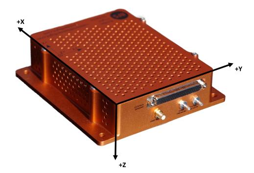
Figure 4: PDAS coordinate system
